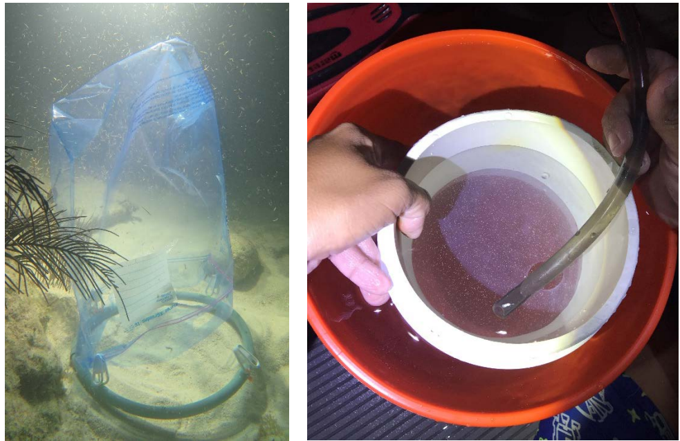
Fig 3. Coral gamete collection device made of weighted hose and large plastic bag (left). In-water sieve used to gently concentrate eggs (right. Photo by CRF).
