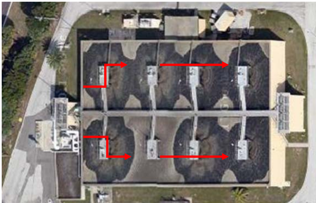
Figure 2 – Current Reactor Configuration at the SWWRF
