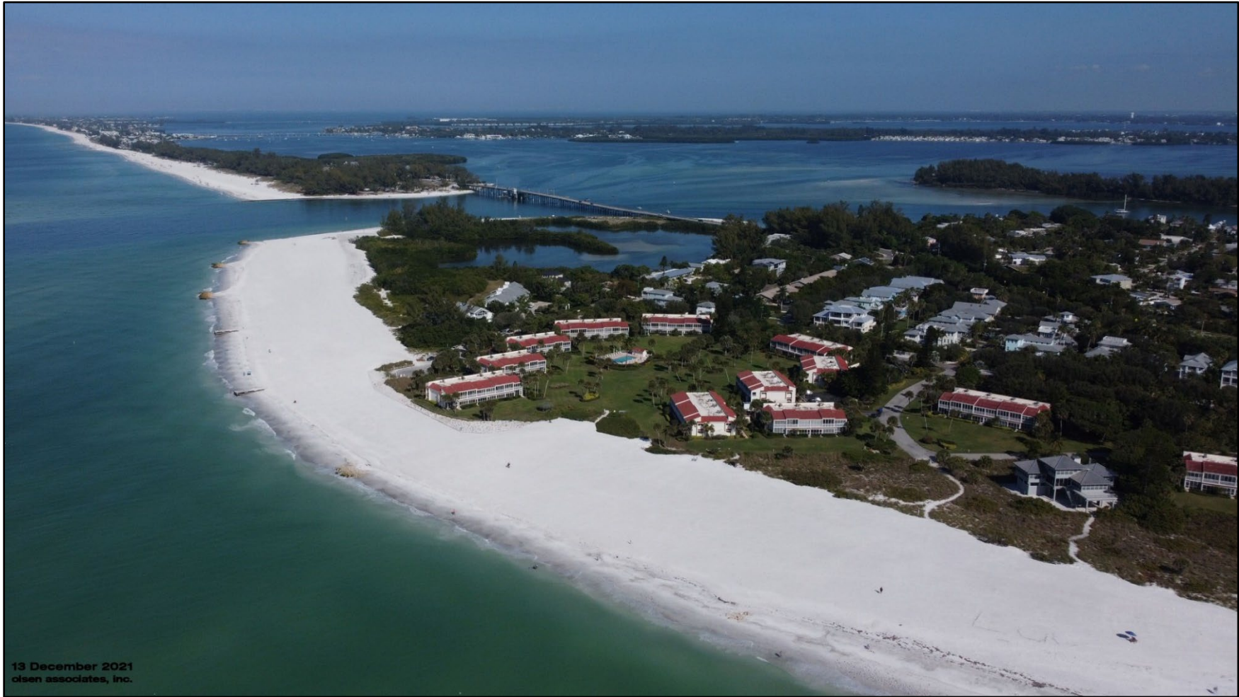
Figure 25: Longboat Pass post-construction showing bypassed material placed to the north at Coquina Beach (R33 to R41) by CPE for Manatee County and south to North Longboat Key (R42 to R44.4) by Olsen Associates for the Town of Longboat Key. Photo courtesy of Al Browder with Olsen Associates, December 2021.
