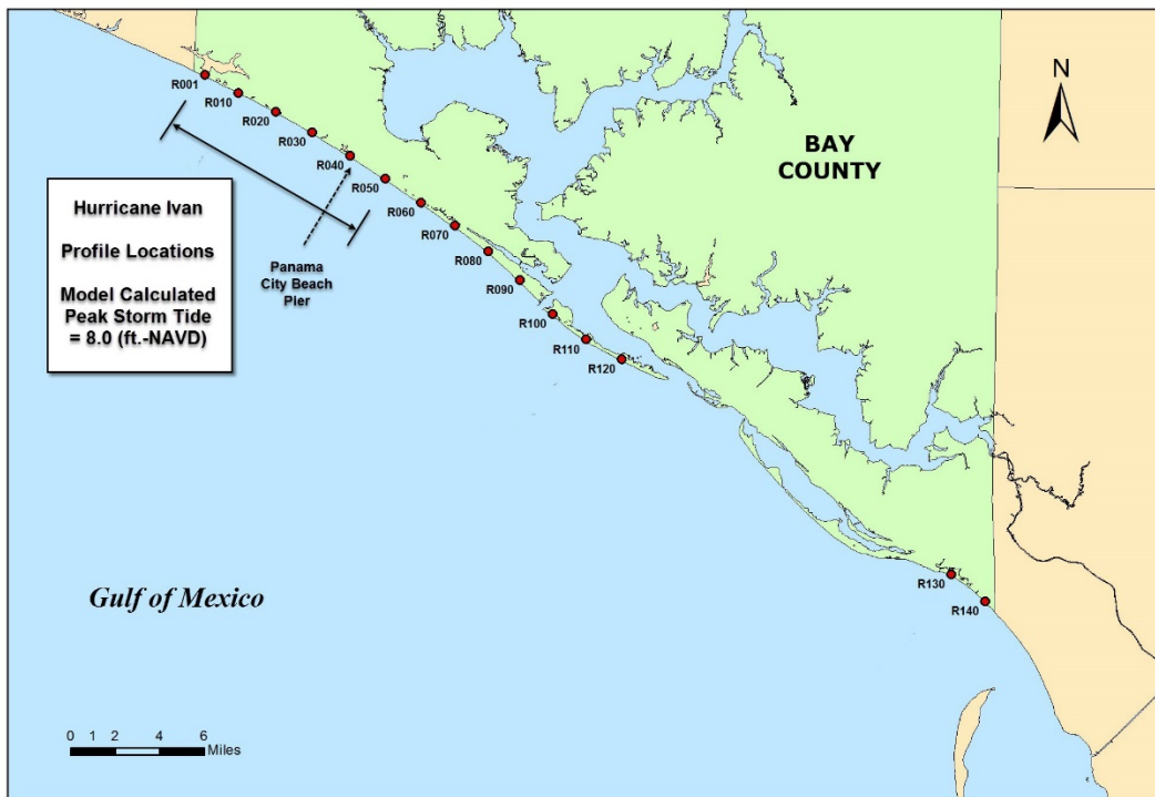
Figure 9: Locations of Profiles and the Calculated Peak Storm Tide Used in SBEACH Calibration.
