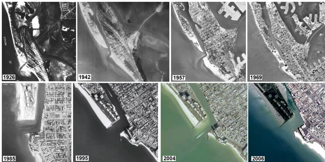
Figure 3. Historical aerial photos of Blind Pass showing both erosion and accretion to the adjacent shorelines (various sources: U.S. Dept. of Commerce; FL Dept. of Transportation; USF-CRL).
