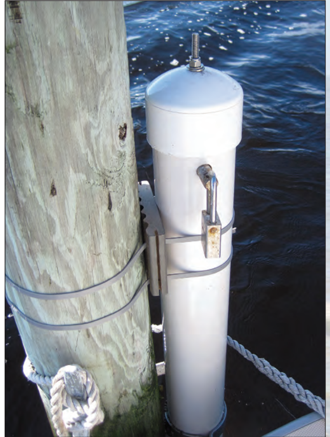
Data sondes are used to collect continuous water quality data in Matlacha Pass Aquatic Preserve.
