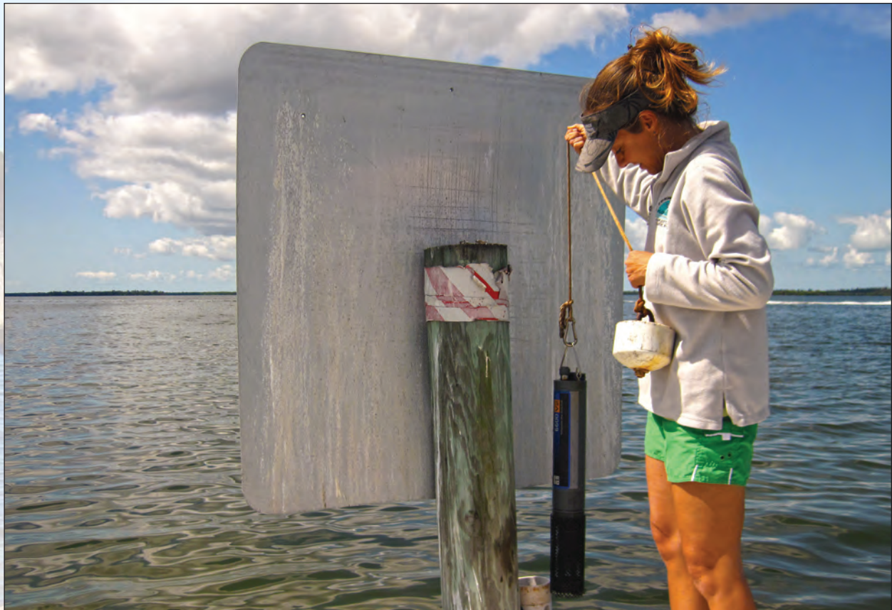
Staff checking on one of the data sondes used to monitor water quality.
