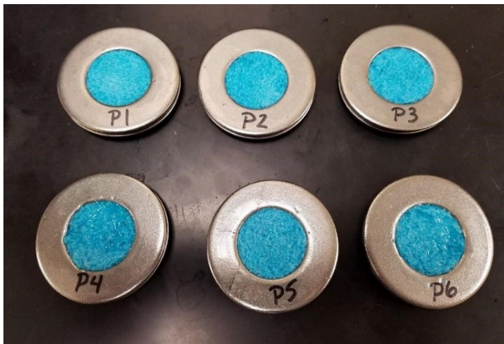
Image-1: Dies Filled with ~1 gram of Ointment for Dissolution Testing in the UV-Vis Spectrometer
