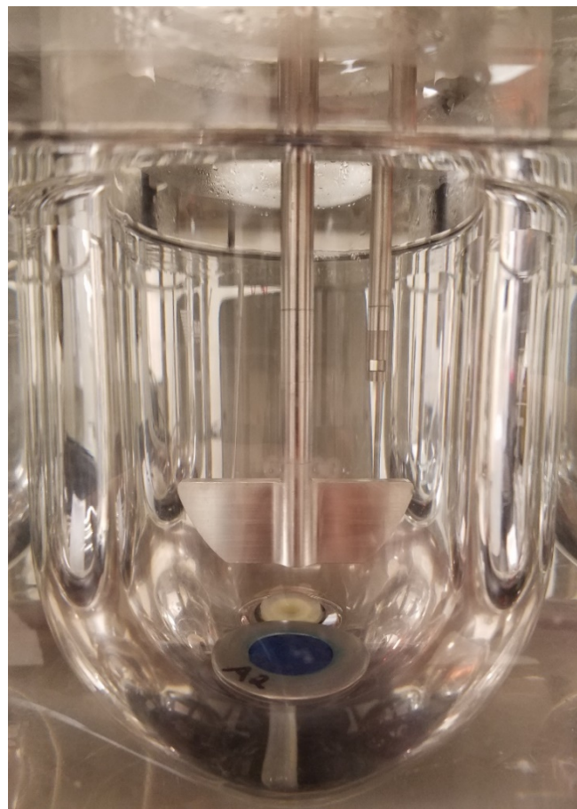
Image-2: 1000 mL UV-Vis Dissolution vessel with Die Cavity Containing ~ 1 gram of Ointment Sample
