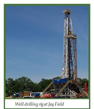
A surface hole is drilled below the base of the underground source of drinking water (typically 1,400 to 2,000 feet deep). Once the specified depth is reached, the drill crew lines the borehole with well casing and cements it in place to prevent wellbore collapse and protect any potential drinking water aquifers. In South Florida, an additional intermediate hole is drilled, cased, and cemented in order to isolate the well from a particularly porous and saline layer known as the "Boulder Zone."
