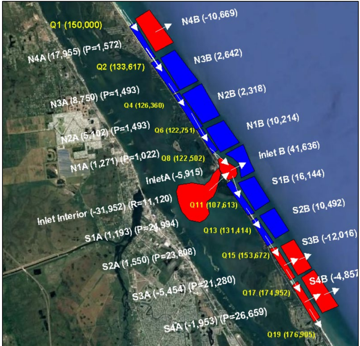
Figure 2: Dr. Zarillo's Summer 2011-2021 bifurcated sediment budget including placement (P) and removal (R) volumes per cell. Blue and red cells correspond with accretion and erosion respectively.
