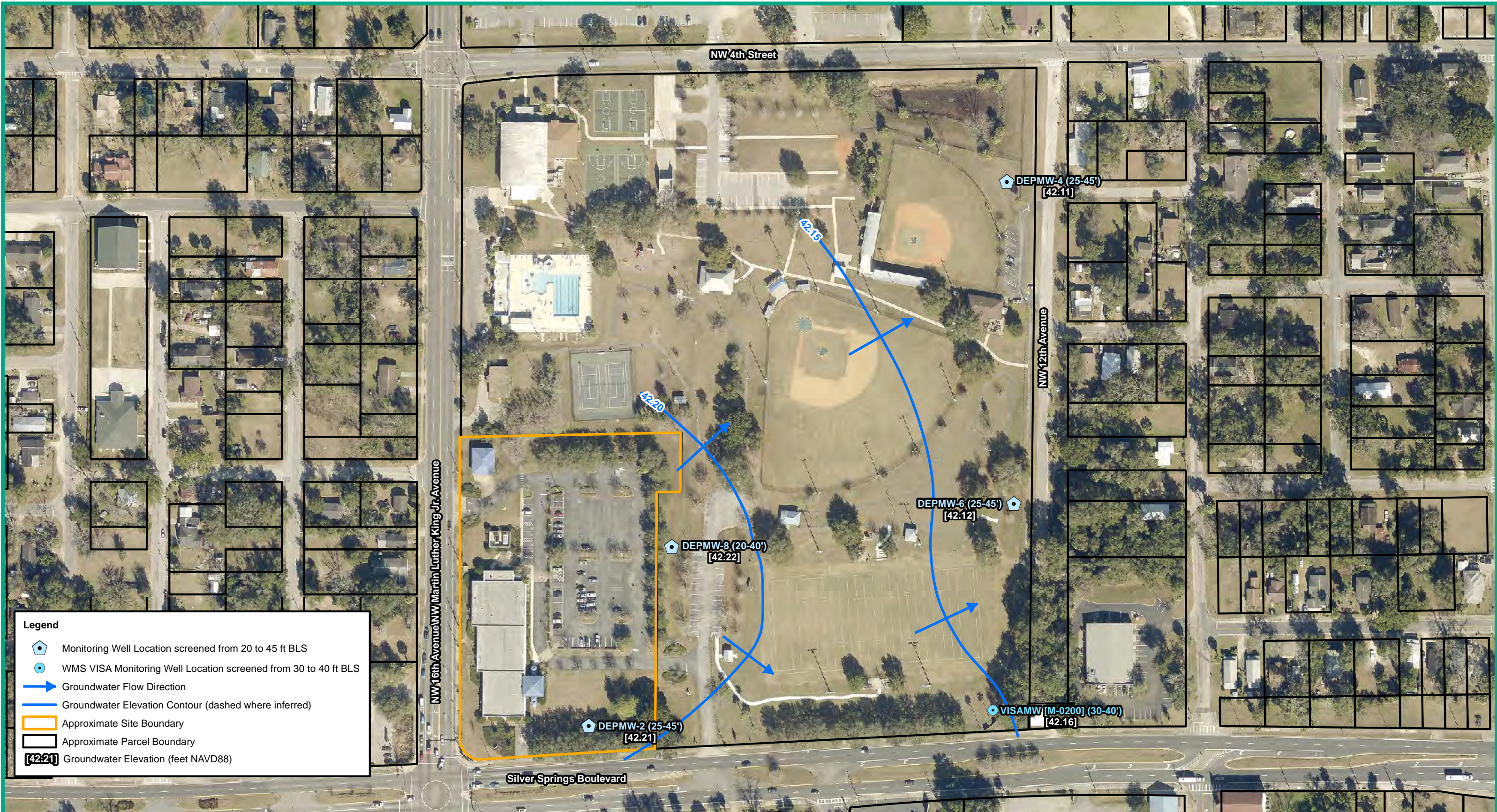
Figure 9 Groundwater Elevation Contour Map from 20 to 45 ft BLS - 28 March 2022 Former Florida State Fire College 1501 West Silver Springs Boulevard Ocala, Marion County, Florida
