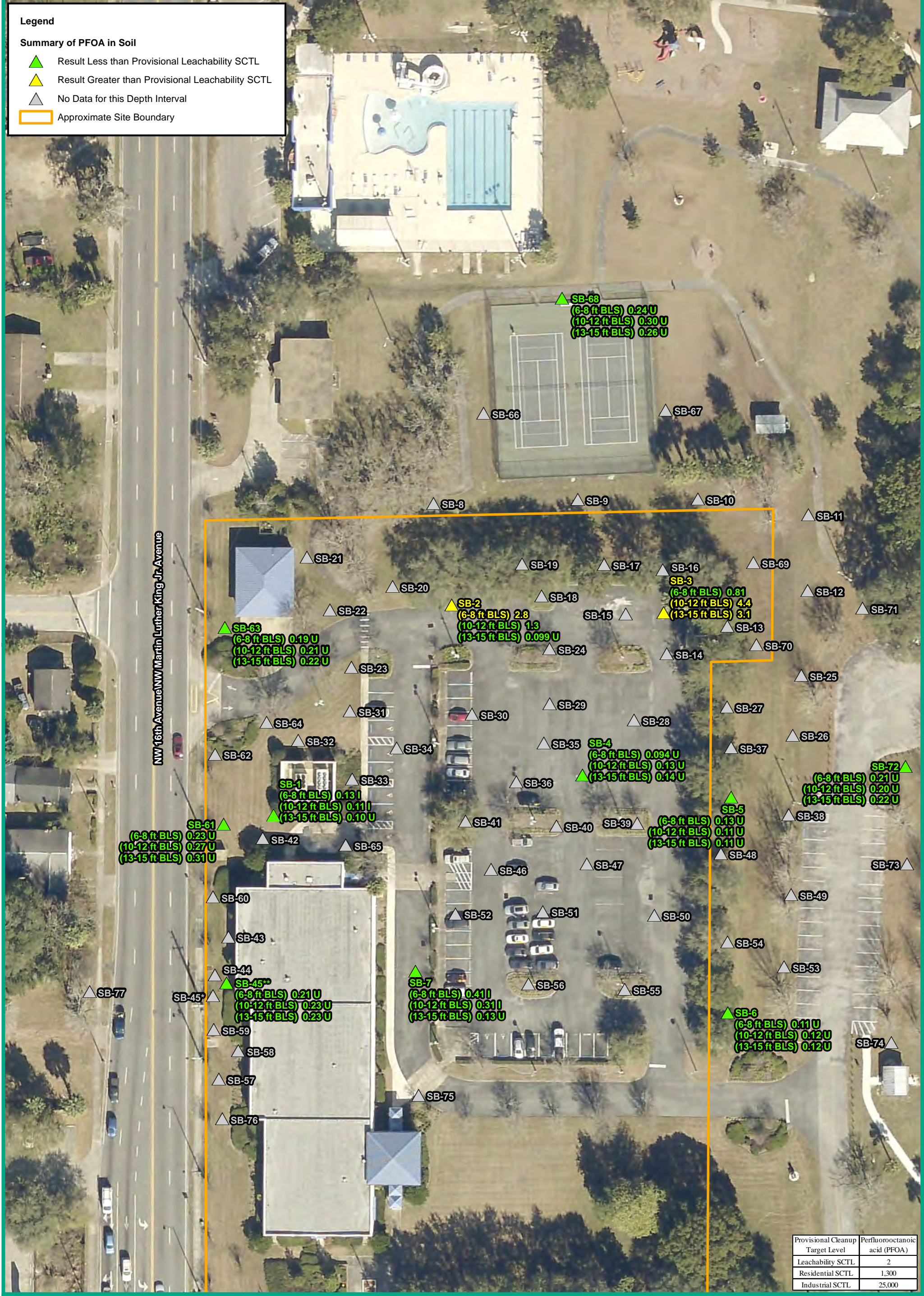
Figure 22 Summary of PFOA in Soil from 6 to 15 ft BLS Former Florida State Fire College 1501 West Silver Springs Boulevard Ocala, Marion County, Florida
