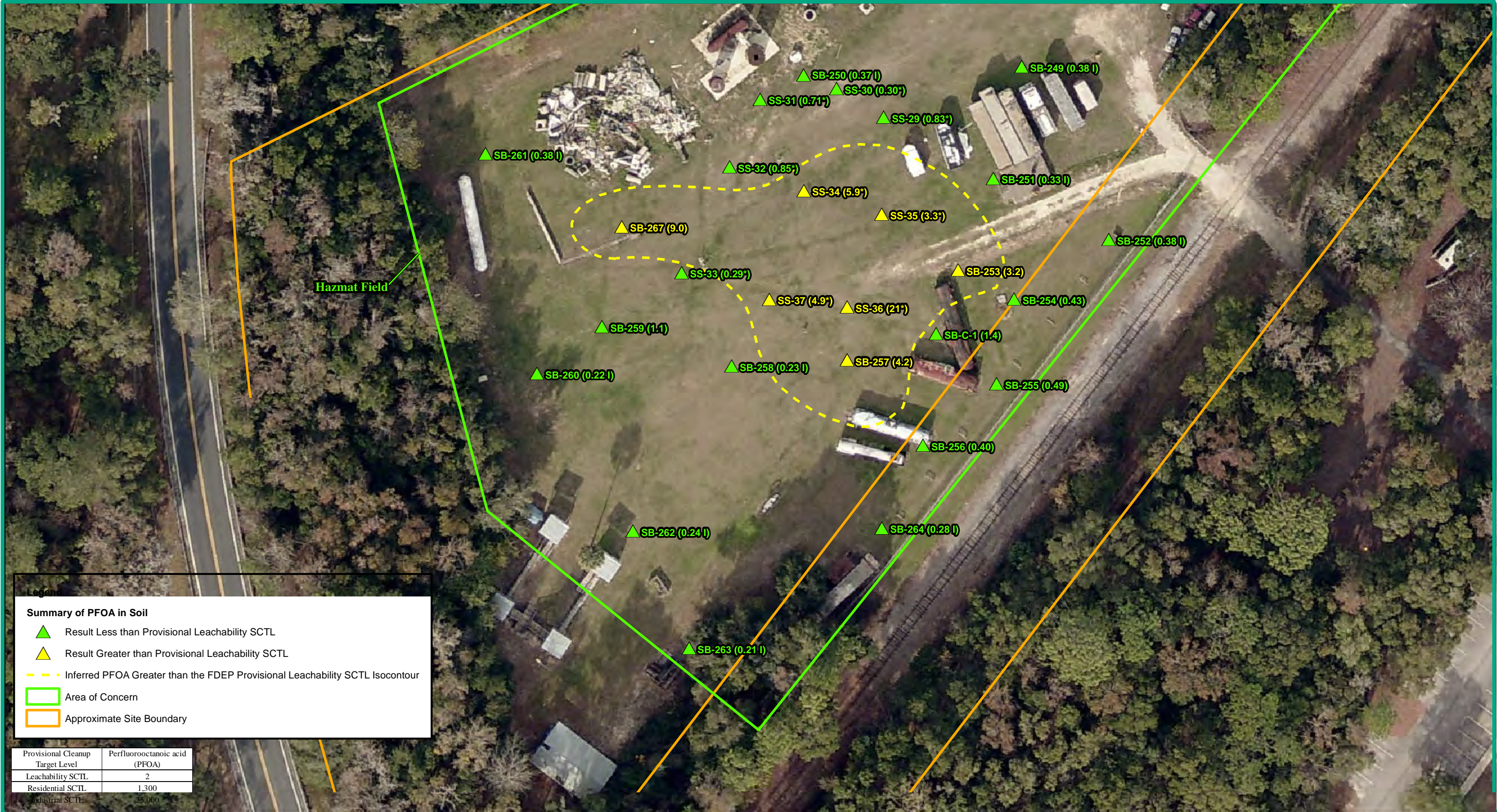
Figure 23 Summary of PFOA in Soil from 0 to 0.5 ft BLS in Hazmat Field Area Florida State Fire College 11655 NW Gainesville Road Ocala, Marion County, Florida
