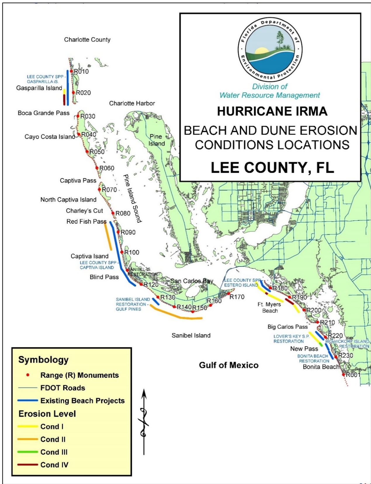
Figure 43. Lee County beach and dune erosion conditions from Hurricane Irma.
