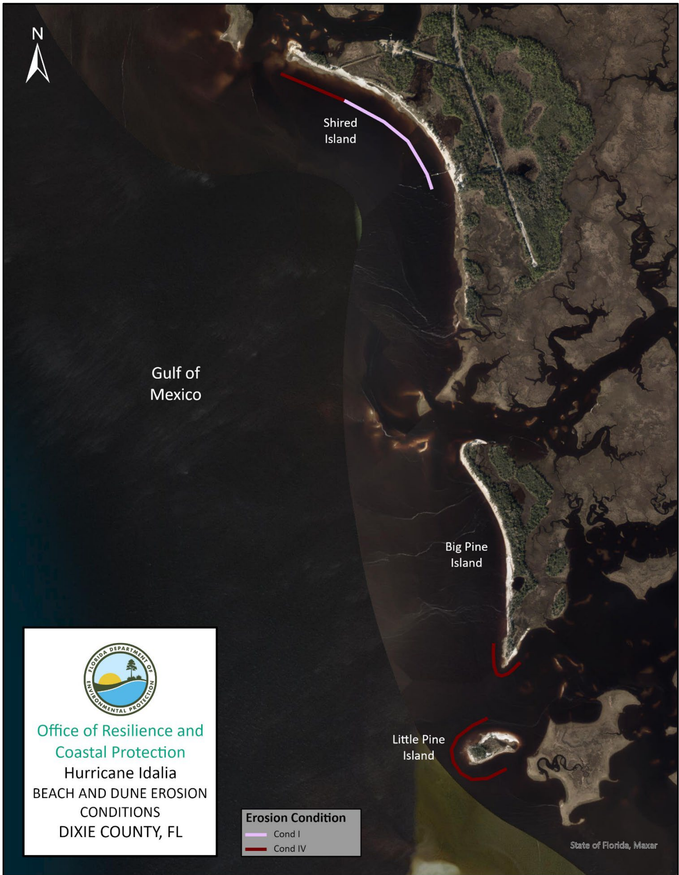
Figure 18. Southern Dixie County Beach and Dune Erosion Conditions from Hurricane Idalia.
