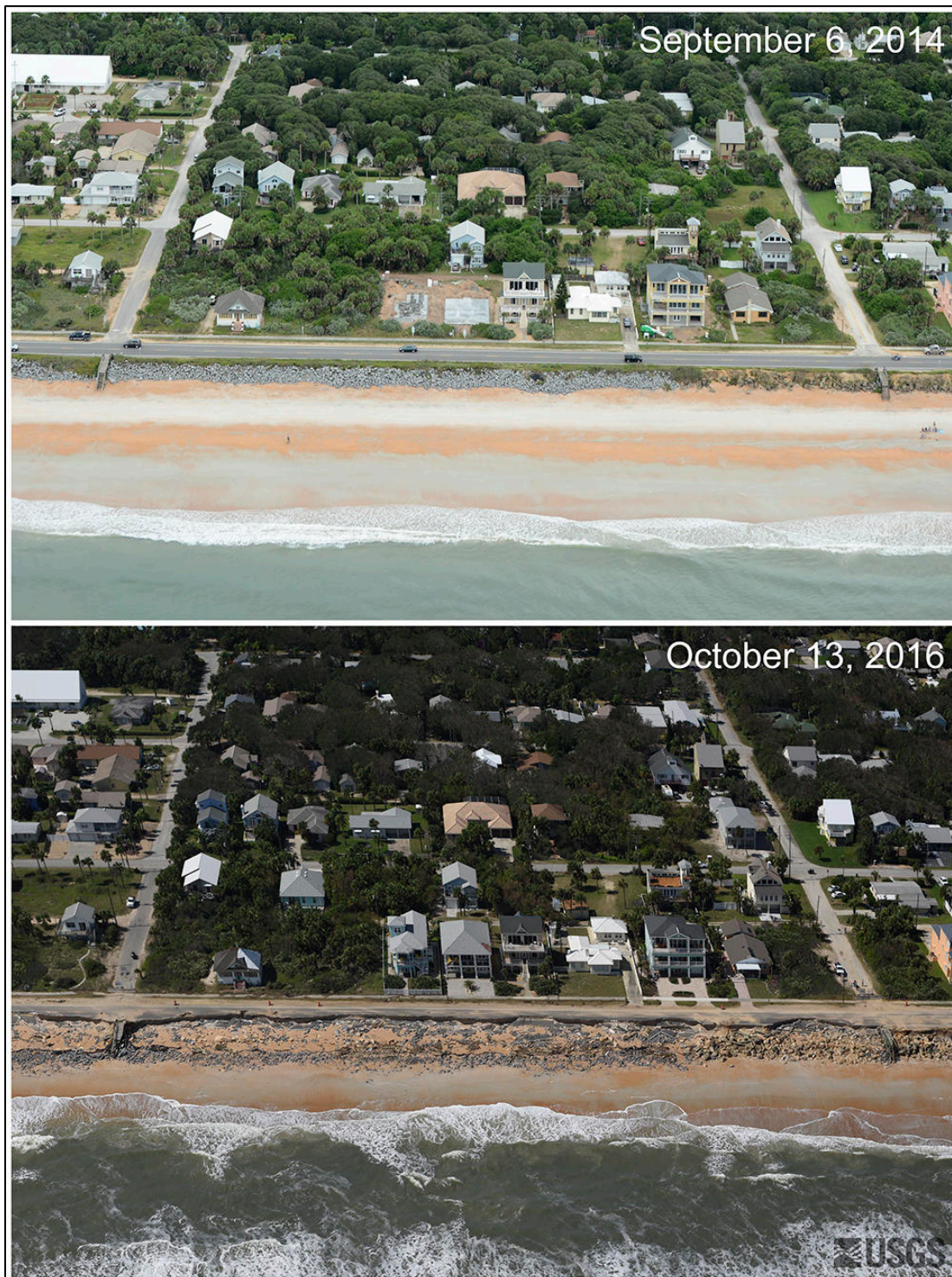
Figure 18d. Before and after photos of Flagler Beach showing rock revetment and State Road A1A destroyed between 14 th St. South and 15 th St. South (R83) [Photos courtesy of U.S. Geological Survey].
