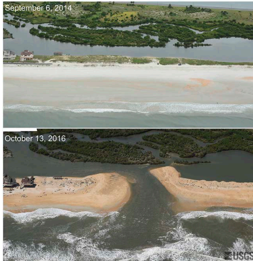
Figure 17f. Before and after photos of barrier breach creating a new tidal inlet at Summer Haven, St. Johns County (R204.5) [Photos courtesy of U.S. Geological Survey].
