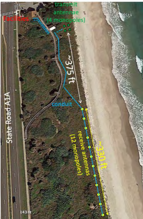
LEFT: Proposed locations for the transmit antenna (green), receive antenna (yellow) and cables (cyan). RIGHT: Land parcel boundaries obtained from the Brevard Co. Property Appraiser ( https://www.bcpao.us/PropertySearch/#/nav/Search ).
