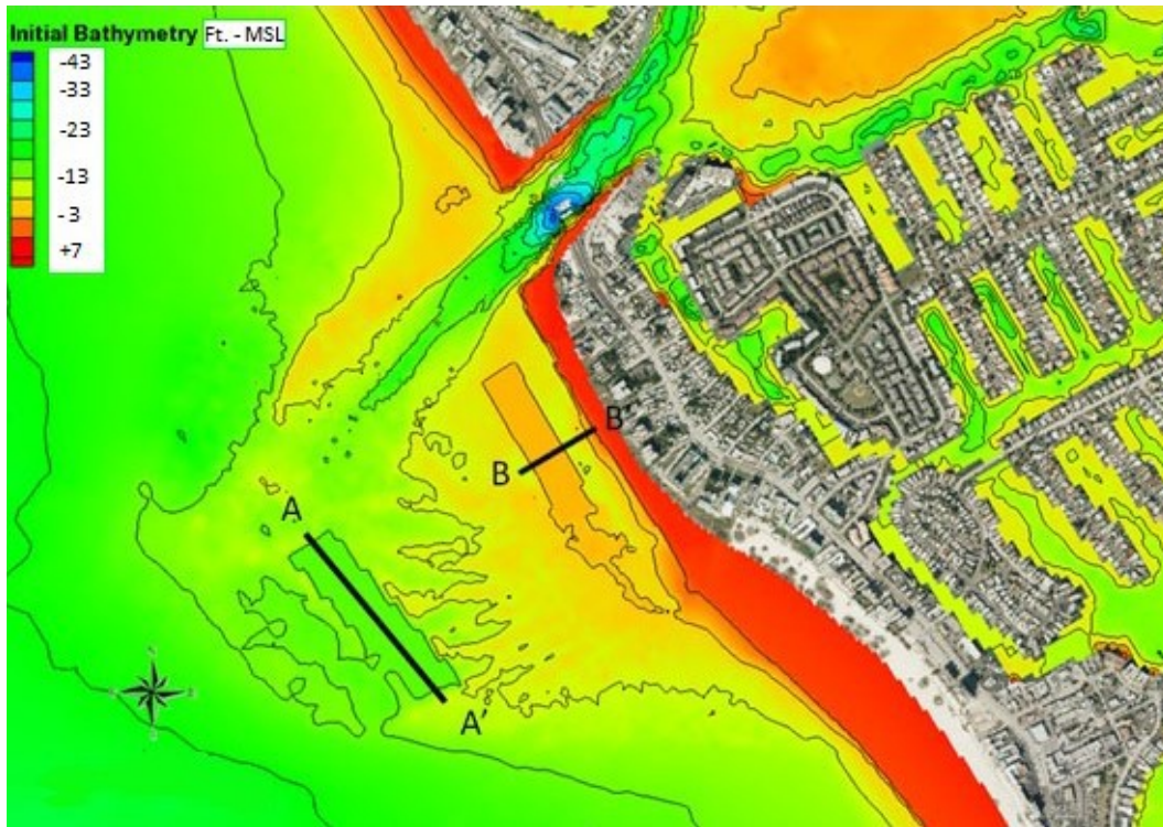
Figure 6. Alternative 3 showing the dredge pit (A-A') and the berm nourishment (B-B') (Wang et al., 2016).
