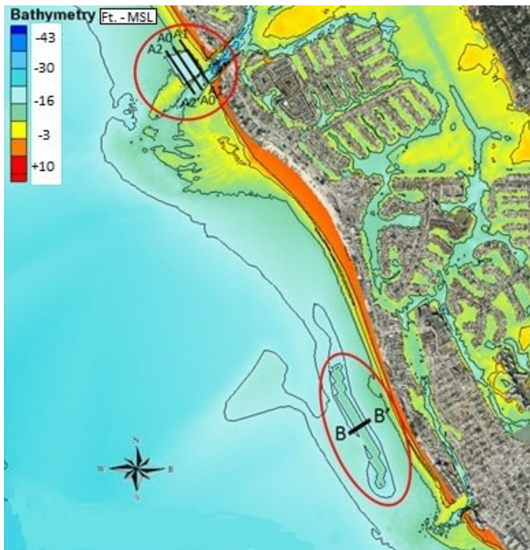
Figure 5. Bathymetry for the Alternative 2 model run. A dredge pit (A-A') is excavated at the channel margin linear bar just north of the John's Pass navigation channel. The sand is placed in an old dredge pit (B-B') seaward of Sunset Beach (Wang et al., 2016).
