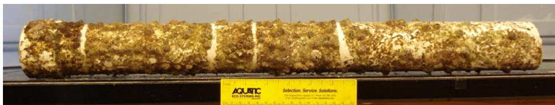
Figure 5. Sediment trap recovered from PE3 in June, 2008, showing heavy colonization by marine organisms. Scrape marks from grazers are evident toward the trap's top (right side of photo). The circumferential bands of bare PVC (above the ruler) were covered by plastic cable ties that secured the trap to its U-post.
