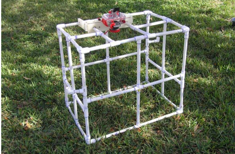
Figure 13: Rigid 0.5 x 0.75 underwater camera framer.
