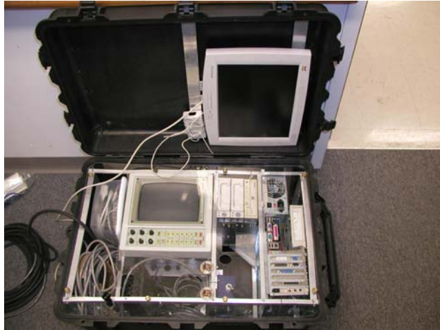
Figure 11: The survey unit consisting of a Suzuki 2025 Echosounder, the various boards associated with the QTC View and Echoplus acoustic ground discrimination systems, and the data collection computer with flat screen. The entire unit is in a waterproof box.
