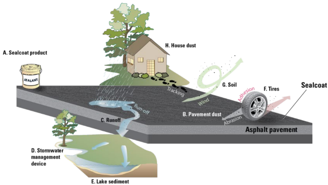
Figure 1-2 PAHs from coal-tar-based pavement sealants. Dried sealcoat products (A), gradually abrade to a powder and become part of the dust on the pavement (B). Pavement dust is transported by rainfall runoff (C) to stormwater management devices (D) or to receiving streams and lakes (E). Pavement dust also adheres to tires (F) that track it onto unsealed pavement, and wind and runoff transport the dust to nearby soils (G). Sealcoat particles tracked into residences can become incorporated into the house dust (H). Graphic from USGS Fact Sheet 2016-3017 .
