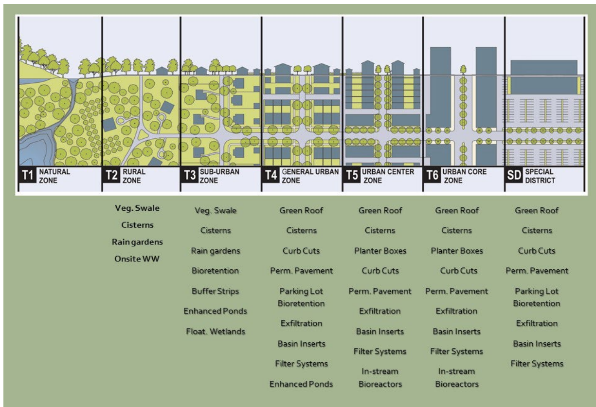
Figure 6-1. Rural to urban transects and suitable LID SCMs. (Graphic by Duany Plater-Zyberk & Company)
