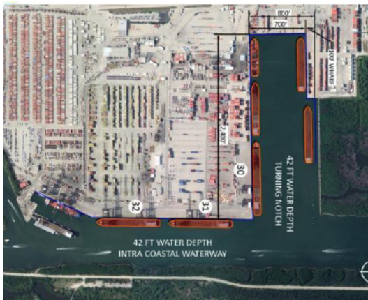
E. Turning notch expansion at current depth of 42ft (Project 1).
