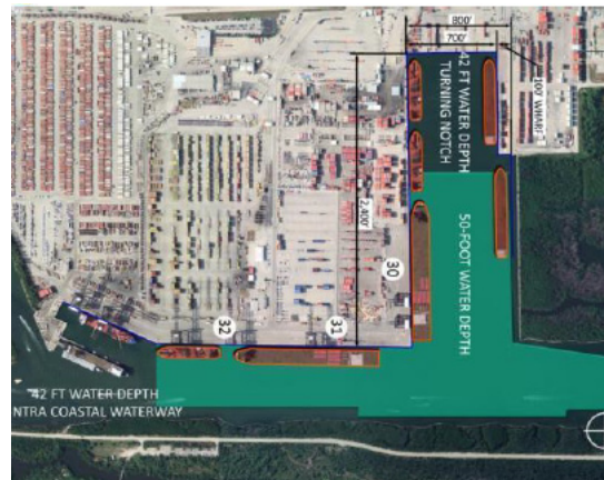
F. Turning notch deepening to 50ft (Project 2).
