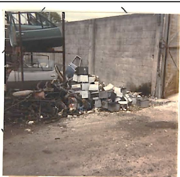
Picture Explanation: BATTERIES IMPROPERLY STORED
