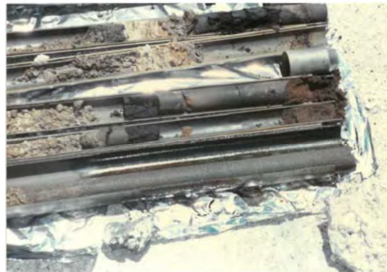
July 1990 SI - MGP waste stained soil cores. West Palm Beach MGP Aka: Florida Public Utilities Inc
