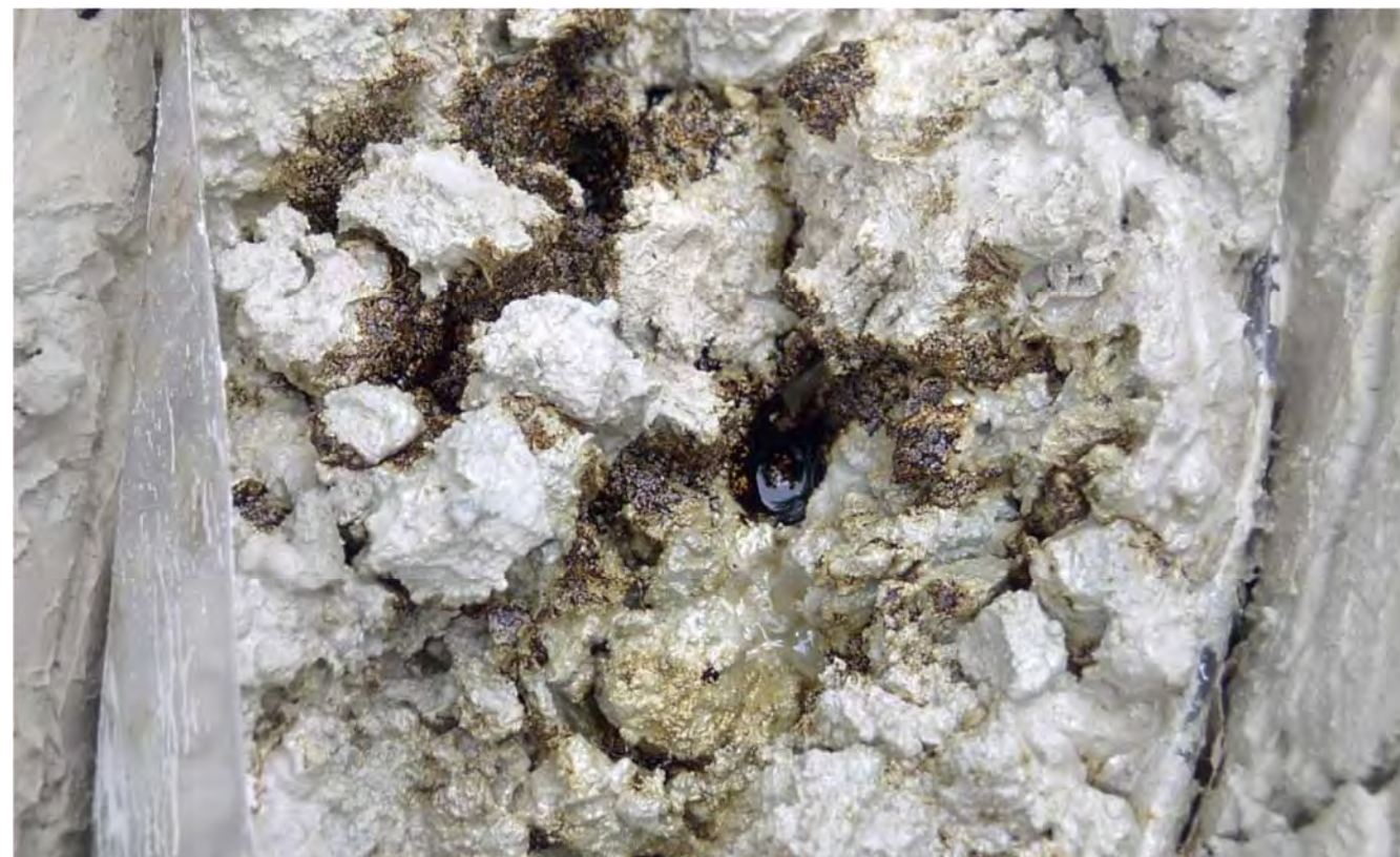
Tampa MGP Rotosonic core sample containing tar NAPL blebs, stringers and pore space saturation in a calcareous clay unit courtesy Arcadis
