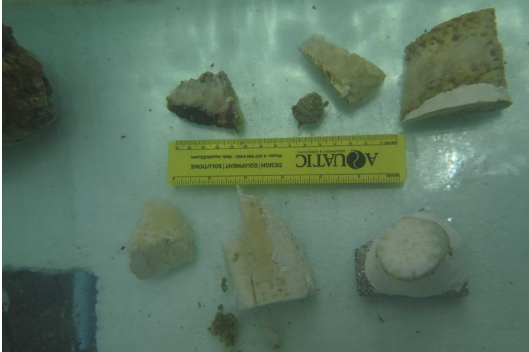
Photo 10. Testing adhesion of CoreRx drug delivery formula on coral skeletons with varying levels of biofilms.
