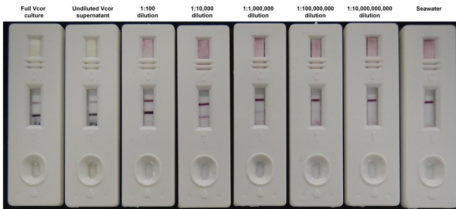
Figure 2. Vibriosis VcpA RapidTest. The immunological assay tests for the presence of the toxin, VcpA, secreted by virulent strains of V. coralliilyticus . A positive test is indicated by two lines, while a negative test is one. The assay is also semi-quantitative with more VcpA (and theoretically more bacteria) indicated by a darker line.
