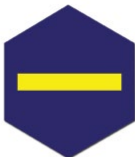
No. 1 Fuel Oil Fill Cover
