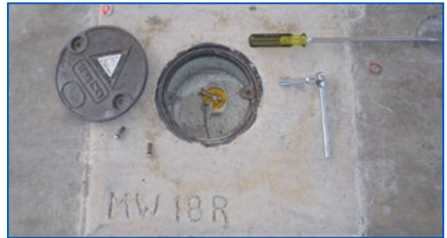
Installed MW with Grout Intact
