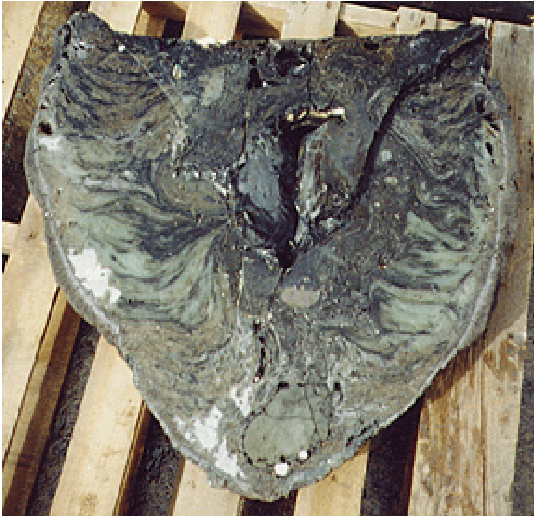
Cross section of a vitrified monolith from the Savannah River Site demonstration.
