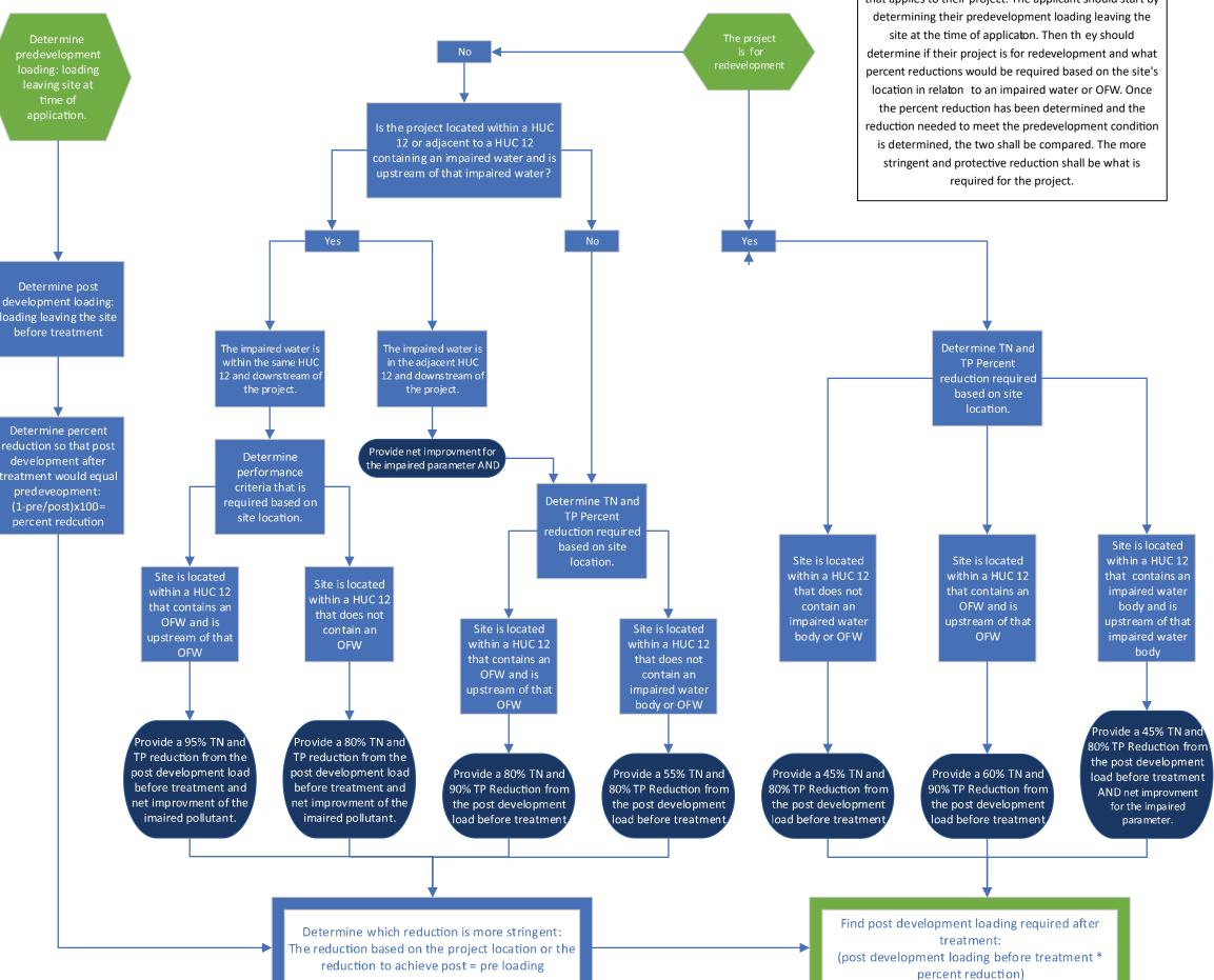
This flow chart describes the path an ERP applicant should take in determining the performance standard that applies to their project. The applicant should start by
