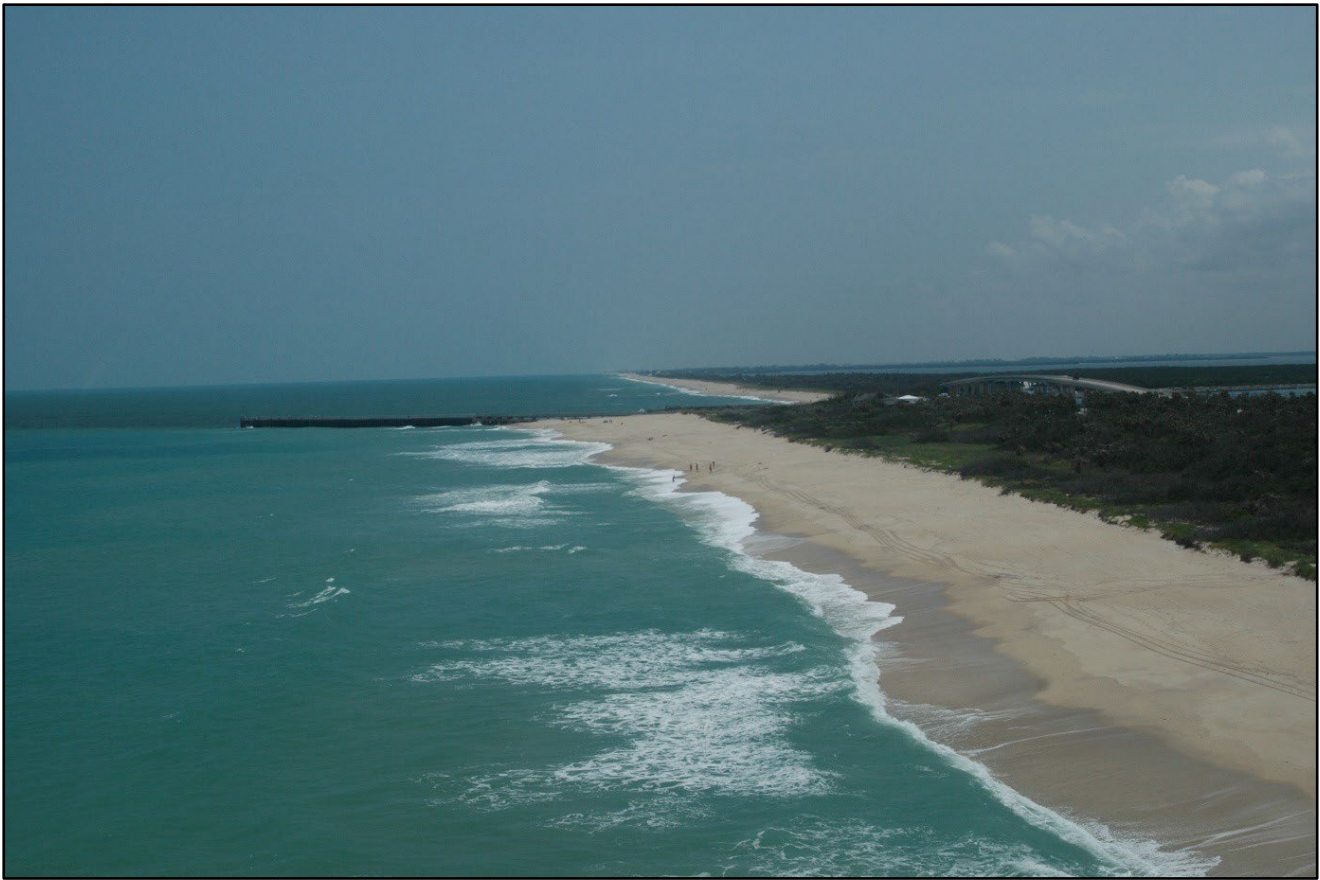
Figure 10. This photo of the Sebastian Inlet from 2005 illustrates how inlets can impede the natural flow of sand along the littoral zone and shows the offset of the coastline on either side of the inlet. The offset is common with altered inlets. DEP project file photo.
