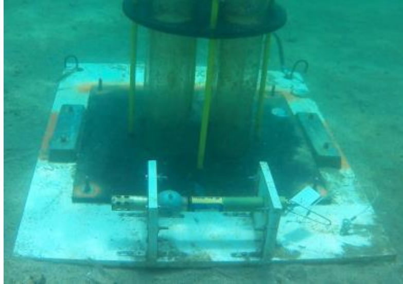
Figure 14: One of the underwater sediment traps with sensors attached that is deployed at the six reef sites.
