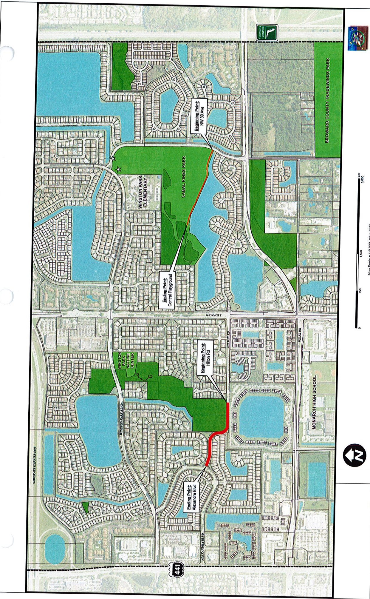
Sabal Pines Trailway Phase I is 12 ft. wide and 1609 ft. long. The Beginning point of the trailway features a trailhead. The halfway point of the trail features a pergola and bicycle rack.
