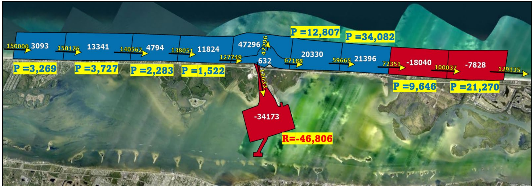
Figure 14. FDEP revisions to the Sebastian Inlet sediment budget. \Delta V values are presented in white with updated placement (P) and removal (R) values from Table 6. Blue and red cells respectively correspond with areas of accretion and erosion.
