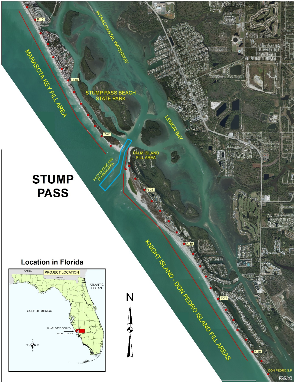
Figure 2. Stump Pass and adjoining beaches showing beach fill placement areas (2013 aerial).
