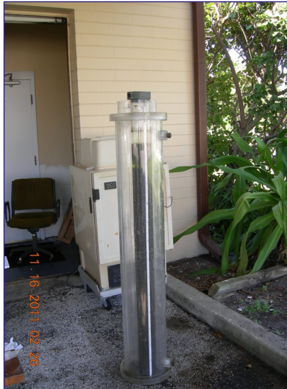
Figure 1. Experimental Steup to Determine the Mixed Liquor Settling Characteristics
