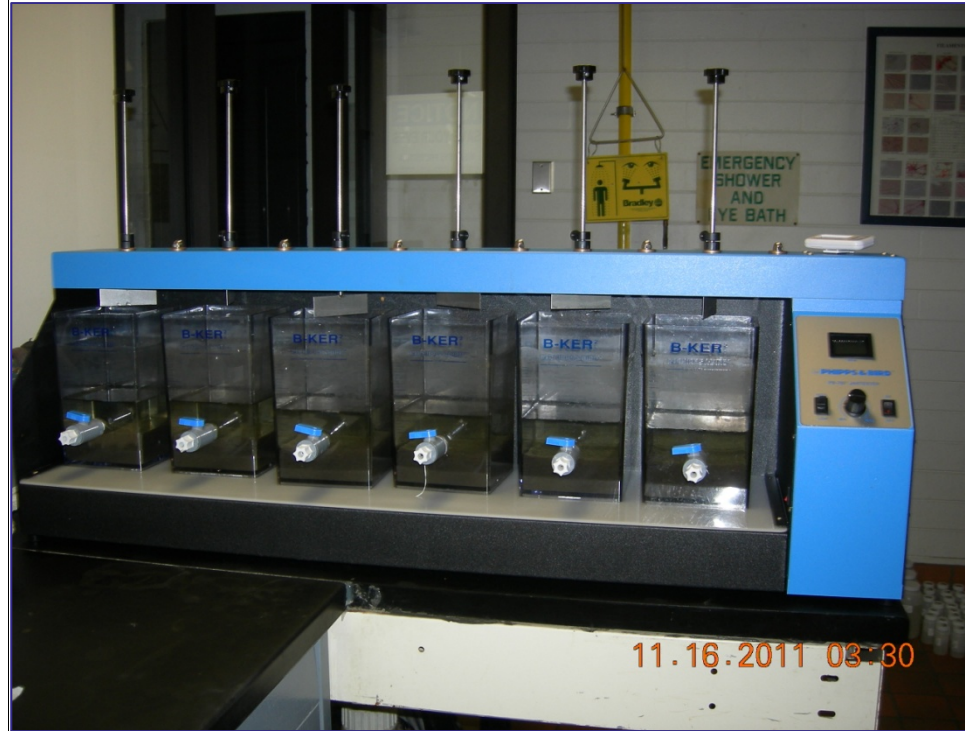
Figure 3. Jar Test Experiment Setup for Determining Flocculation Characteristics
