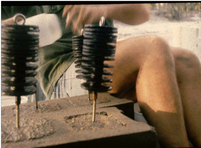
Figure 2. Photo of Hester-Dendy samplers used for determining the Shannon-Weaver diversity index.
