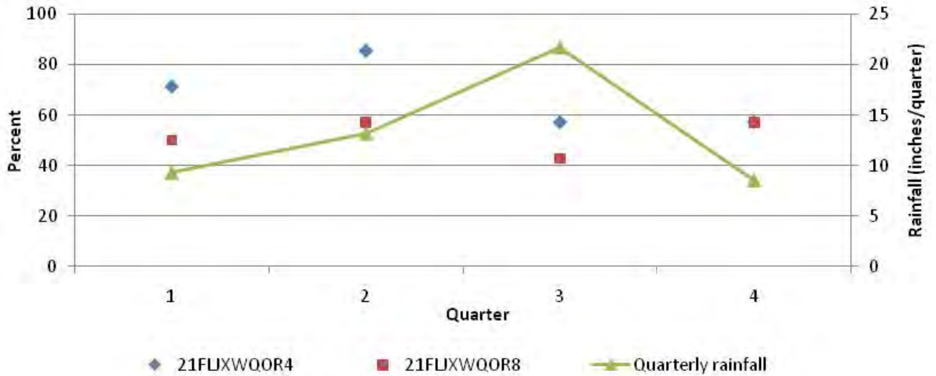
Figure 5.5. Fecal Coliform Exceedances and Rainfall at Stations 21FLJXWQOR8 and 21FLJXWQOR4 in Fishing Creek (WBID 2324) by Season during the Cycle 2 Verified Period
