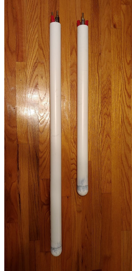
Suction Lysimeter (SL)
