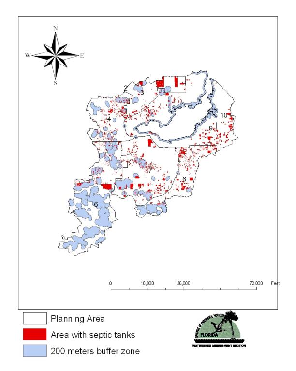
Figure 4.7. Areas with septic tanks, areas within 200 meters of any receiving waters that discharge to Lake Jesup, and planning areas
