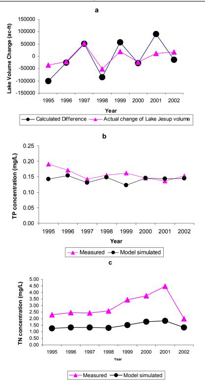
Figures 5.4-a, 5.4-b, 5.4-c. Results for flow and TN and TP calibrations, using the Bathtub model, 1995–2002
