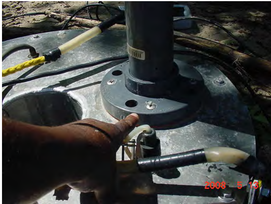
Figure H-6: Lake Munson at public boat landing showing closeup of SOD chamber and YSI; meter inserted into chamber on 5-13-2008
