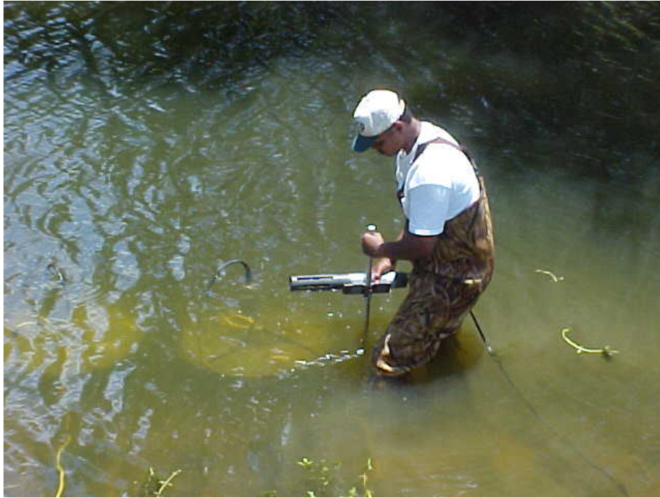
Figure H-3: Munson Slough upstream culverts SOD chambers deployed on 5-20-2008
