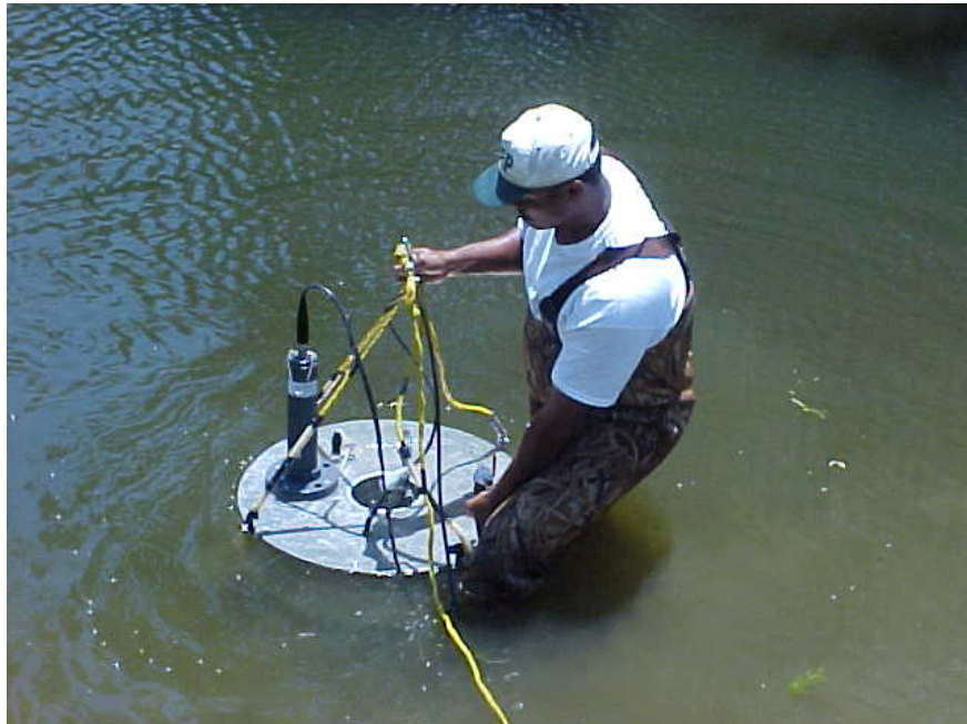
Figure H-2: Munson Slough upstream culverts deploying SOD chamber on 5-20-2008
