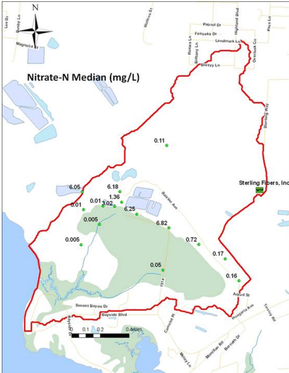
Figure C.5. Judges Bayou Wells Median Nitrate-N (mg/L)
