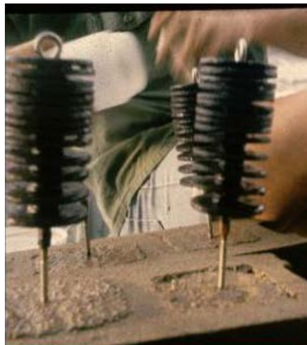
Figure 3-2. Photo of Hester-Dendy samplers used for determining the Shannon-Weaver diversity index.
