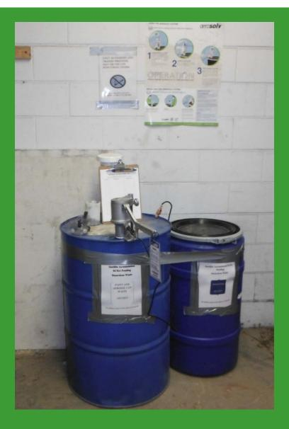
The project used an aerosol can puncturing system to manage its can waste.
